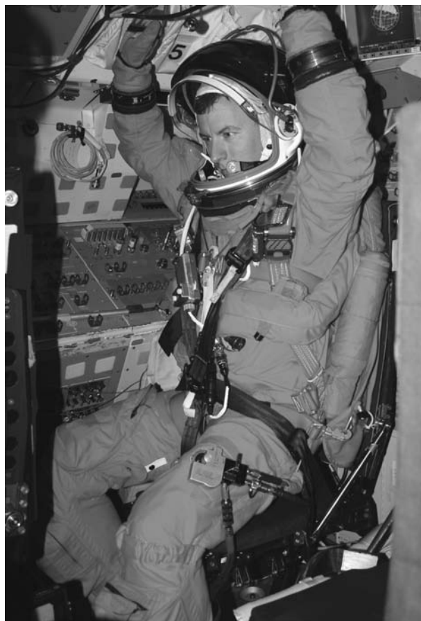
FIGURE 4-18 This five-point restraint harness is currently in use in the space shuttle. Similar designs are found in both military and civilian aircraft (NASA).
